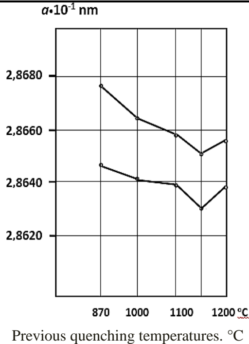
Fig. 2. Change in the grating period of steel U8A depending on the temperature of Previous quenching and intermediate tempering
