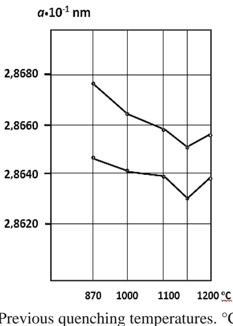
Fig. 2. Change in the grating period of steel U8A depending on the temperature of Previous quenching and intermediate tempering
