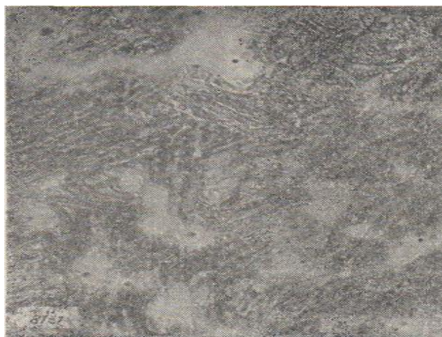
Fig. 1. Microstructure of deposited metal of 25X5ΦMC type (etching with nitric acid, X900)
